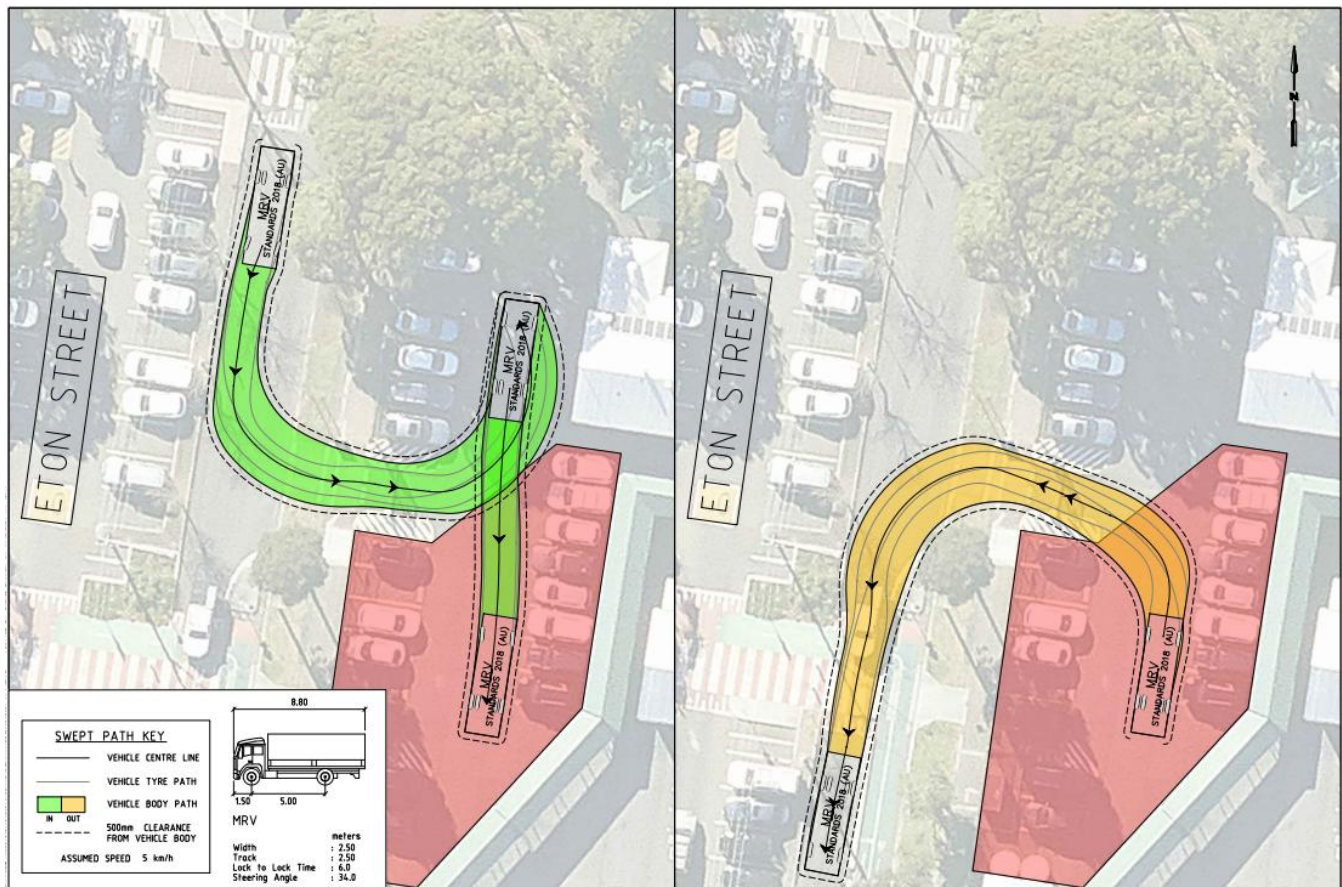
Figure 19: Swept path for construction vehicles (MRV)
